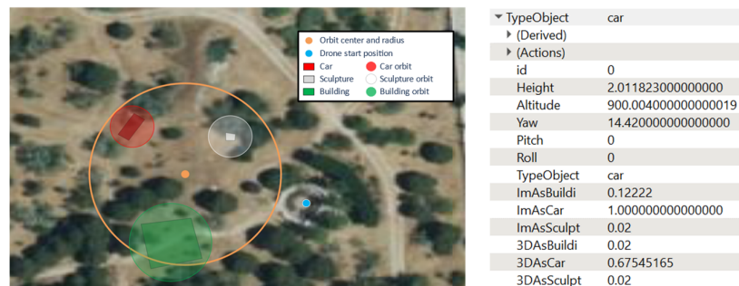
Figure 7 – Orbits and detected objects in GIS (left). Metadata of car GIS layer (right)
